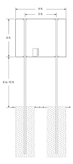
Once you have verified the positions of the posts and the size of the footings, you are ready to dig your holes, pour your concrete, and set your posts. There are several techniques for ensuring proper alignment of the posts. Typically installers will construct a temporary wooden support frame to hold each post in place while the concrete sets. Having plumb posts in the proper position is the key to a smooth mechanical installation.
